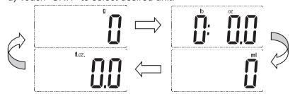
**Note**: When finishing selecting unit, you may start to weigh according to the weighing procedure below. If there is not any operation and the weight is steady in weighing mode, the scale will turn off automatically after about 60s.
