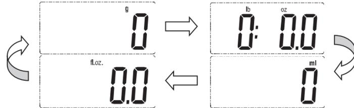
**Note:** When finishing selecting unit, you may start to weigh according to the weighing procedure below. If there is not any operation and the weight is steady in weighing mode, the scale will turn off automatically after about 60s.
