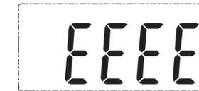
c) Negative weight indication. It will be shown when taking the weight from the platform, under “Tare” setting.
