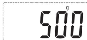
**Note:** If there is not any operation and the weight is steady in weighing mode, the scale will turn off automatically after about 60s.
