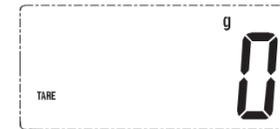
**Note:** “TARE” will be displayed only when the weight of the container is over 600g. And you can use the tare function for many times in one weighing process.
