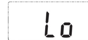
b) Overload indication. Please remove the weight on the scale to protect the loadcells.
