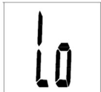
b) Overload indication. Please remove the weight on the scale to protect the loadcells.
