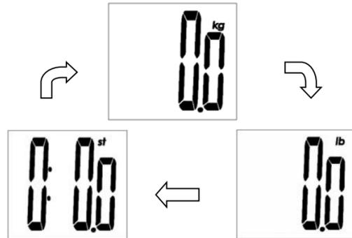
**Note:** Please put the scale on flat hard ground when finishing selecting unit. Wait for a few seconds, then you may start measuring according to the measuring procedure below. If there is not any operation in weighing mode, the scale will turn off automatically after about 10s.
